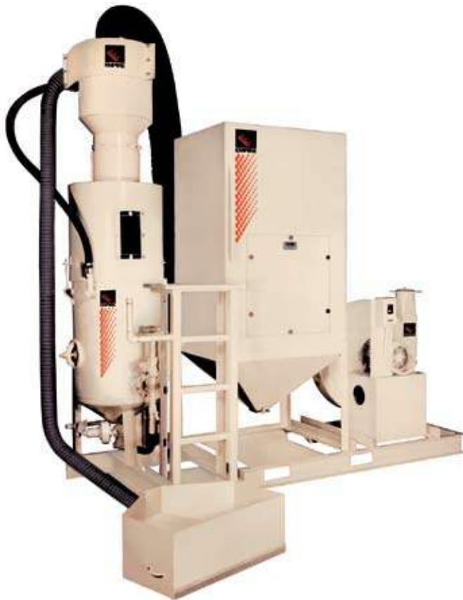
PRS system offers an economical alternative to a full blast room for limited-use operators. In addition to pneumatically collecting media, the unit recycles and cleans abrasives through a cyclonic reclaimer attached to a media-filtration system.
