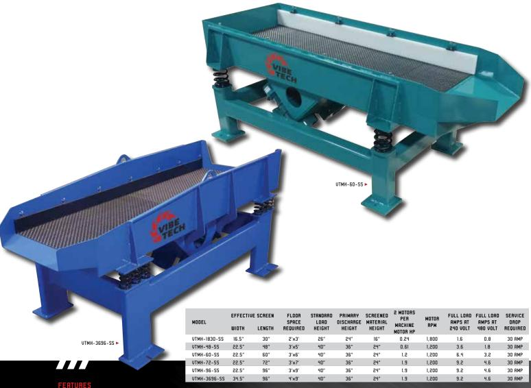
Shaker screeners are an integral part of any mass finishing product line, because they are the most effective way of separation. In the mass finishing industry, shaker screeners, are used for multiple reasons.
